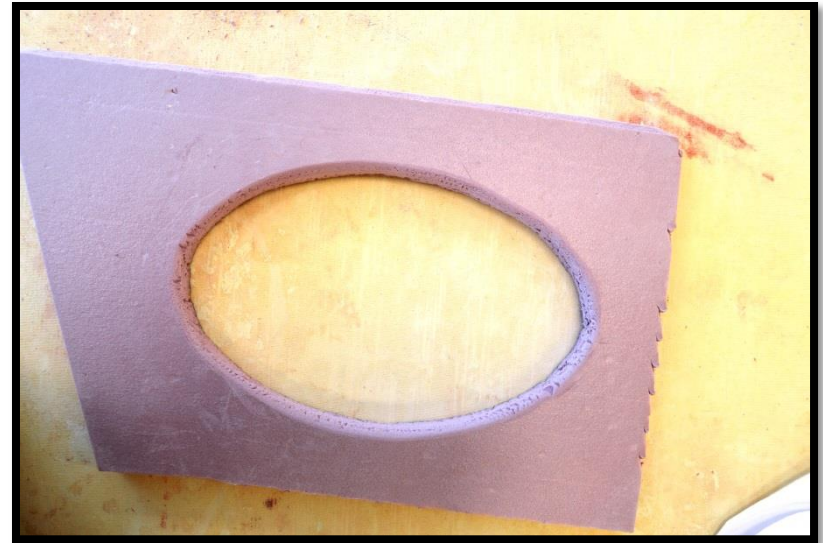
Slump Cut from Insulation Foam.
